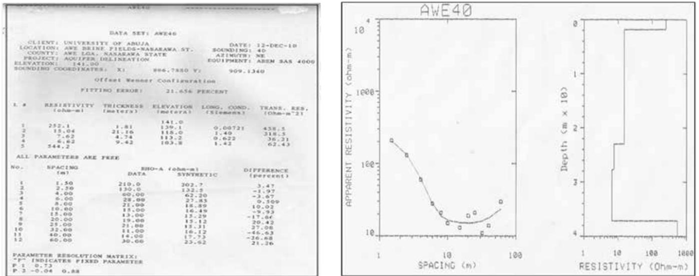
Figure 4b: A typical interpreted 1D resistivity data of VES 40
