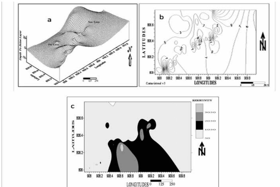
Figure 5: (a) Thickness of The First Layer (b) First Layer Isopach (Isothickness) Map (c) Isoresistivity Zoning map of the upper layer
