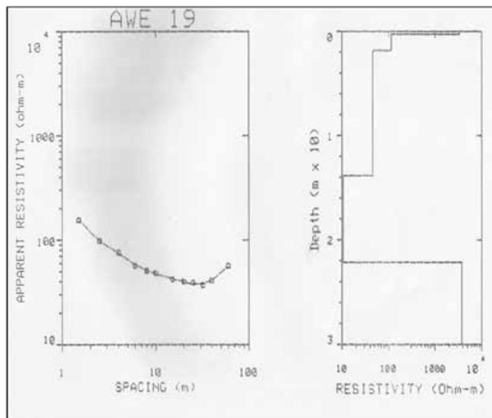
Figure 4a: A typical interpreted 1D resistivity data of VES 19
