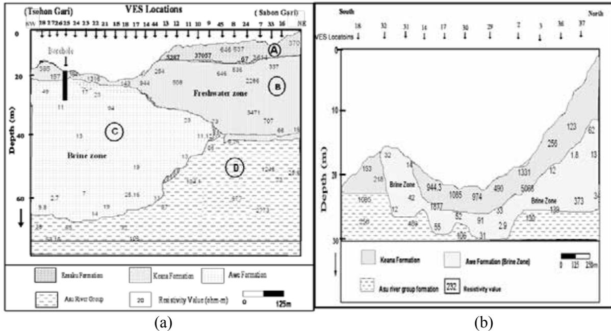
Fig: 8:(a) Geoelectric section along first survey profile (b) Geoelectric section along second survey profile
