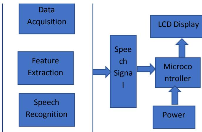
Figure 1: Architecture of the developed speech recognition-based door lock security system
