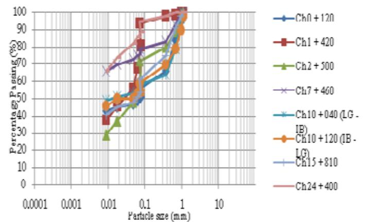
Figure 2: Particle Size Distribution (Stable sections)
